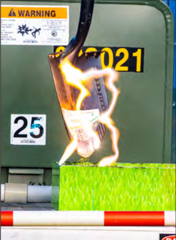
Different items were tested for their conductivity including a shovel, boot, stick, and glove. The shovel, boot, and wooden stick are all touching a ground simulation activated by electricity to simulate what would happen if these items touched the ground. The glove shows the danger of touching metal, like a metal car door, that is activated by live lines. Each of these instances would kill a person.
