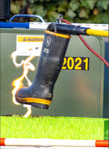
Different items were tested for their conductivity including a shovel, boot, stick, and glove. The shovel, boot, and wooden stick are all touching a ground simulation activated by electricity to simulate what would happen if these items touched the ground. The glove shows the danger of touching metal, like a metal car door, that is activated by live lines. Each of these instances would kill a person.
