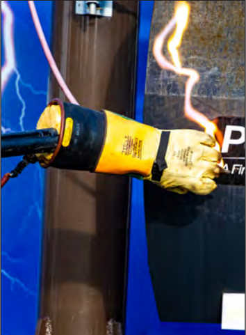
Different items were tested for their conductivity including a shovel, boot, stick, and glove. The shovel, boot, and wooden stick are all touching a ground simulation activated by electricity to simulate what would happen if these items touched the ground. The glove shows the danger of touching metal, like a metal car door, that is activated by live lines. Each of these instances would kill a person.
