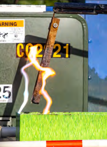
Different items were tested for their conductivity including a shovel, boot, stick, and glove. The shovel, boot, and wooden stick are all touching a ground simulation activated by electricity to simulate what would happen if these items touched the ground. The glove shows the danger of touching metal, like a metal car door, that is activated by live lines. Each of these instances would kill a person.
